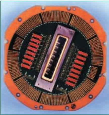
Figure 1. Probe cards for higher pin counts have to accommodate higher pad density where pad pitches are becoming finer and finer.
