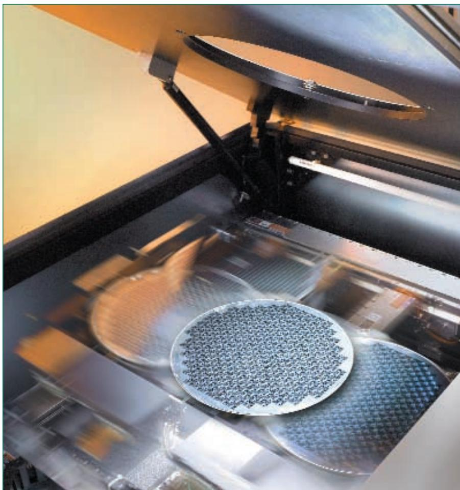
This is an interior view of a highly automated wafer probing system.
